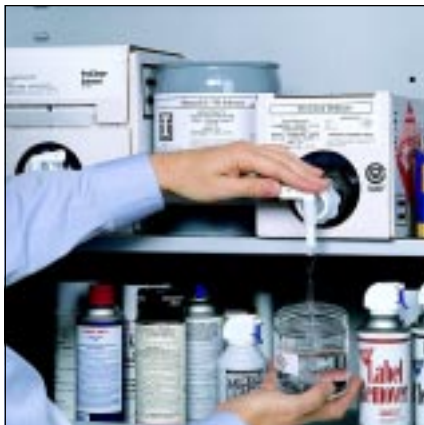
◀ Techs like these rugged cardboard "cubitainers" because they eliminate lifting heavy pails of solvent, avoiding spills.
